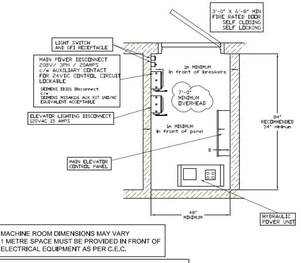
MACHINE ROOM CANNOT CONTAIN ANY MACHINERY, CONTROL PANELS, DUCTING, WIRING OR PIPING THAT IS NOT DIRECTLY INVOLVED WITH THE ELEVATOR
